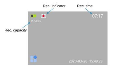
The recording capacity counter indicates the maximum duration of recording available to make. After the memory is full, users needs to manually clear the memory space for future storage, either through the on-board touch screen or using a computer.
